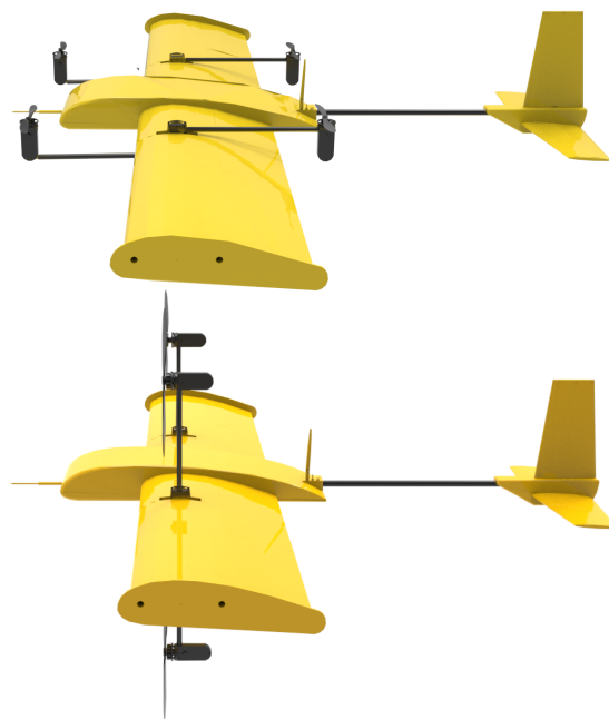
Figure 1. 3D renders of the VTOL UAV both in copter mode (top) and plane (bottom) mode.
