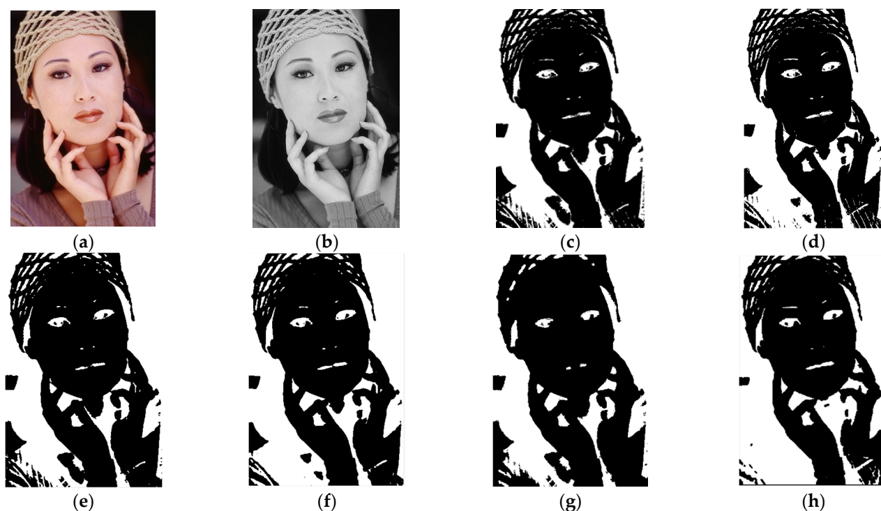
Figure 4. Segmentation of the human face. (a) Original, (b) gray scale, (c) GMM, (d) FCM, (e) FFCM, (f) FLICM, (g) FRGMM and (h) ours. (Adapted from Berkeley dataset, 302003).
