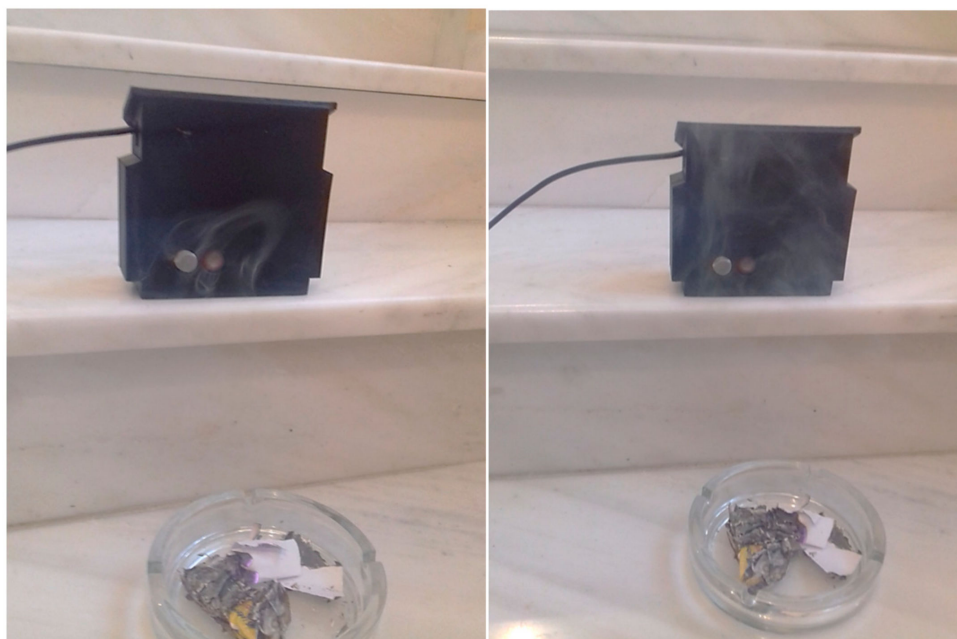
Figure 8. Physical triggering of sensor node 1 by burning a piece of paper.
