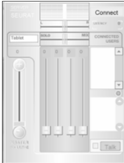
Figure 4. GUI from Tanaka's system for PDAs [18], based on volume-controlled mixing of network transmitted music streams.
