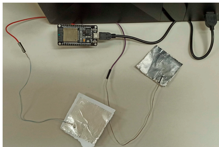
Figure 5. Connection of our capacitive sensors with an ESP32 microcontroller.
