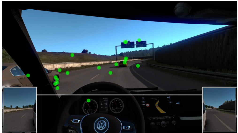
Figure 4. Moment in Video 3 where most participants attended to the windshield (Baseline Task). The green markers represent the gaze coordinates of individual participants. White lines are drawn around the AOIs.
