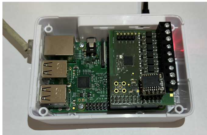
Figure 8. Raspberry Pi 3 equipped with a SensFloor ® hat.
