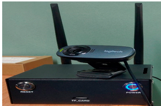
Figure 2. Assembled Jetson-Nano-based smart camera device.
