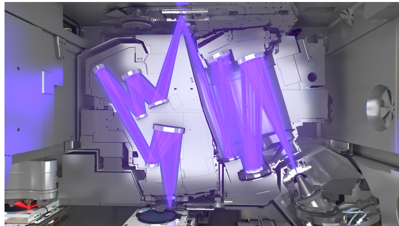
Figure 2. This sequence shows the full light path from the EUV source to the silicon wafer. The light is generated in the source ( bottom-right ), sent into the illuminator ( mid-right ) which controls the light beam, reflects off the mask with the chip pattern ( top ), before being focused on the projection optics ( mid-left ) and exposing the wafer ( mid-bottom ) (Figure based on image (c) ASML).
