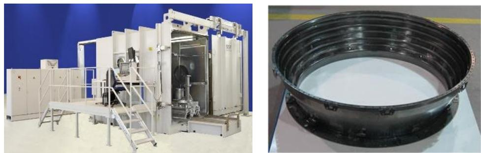
**Figure 7.** High-energy beam electron welding equipment and air inlet casing part.
