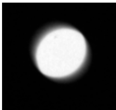
Figure 4. A cropped X-ray radiography image showing the edge effect due to the geometry of the cylindrical flat-bottom hole and the X-ray beam divergence.
