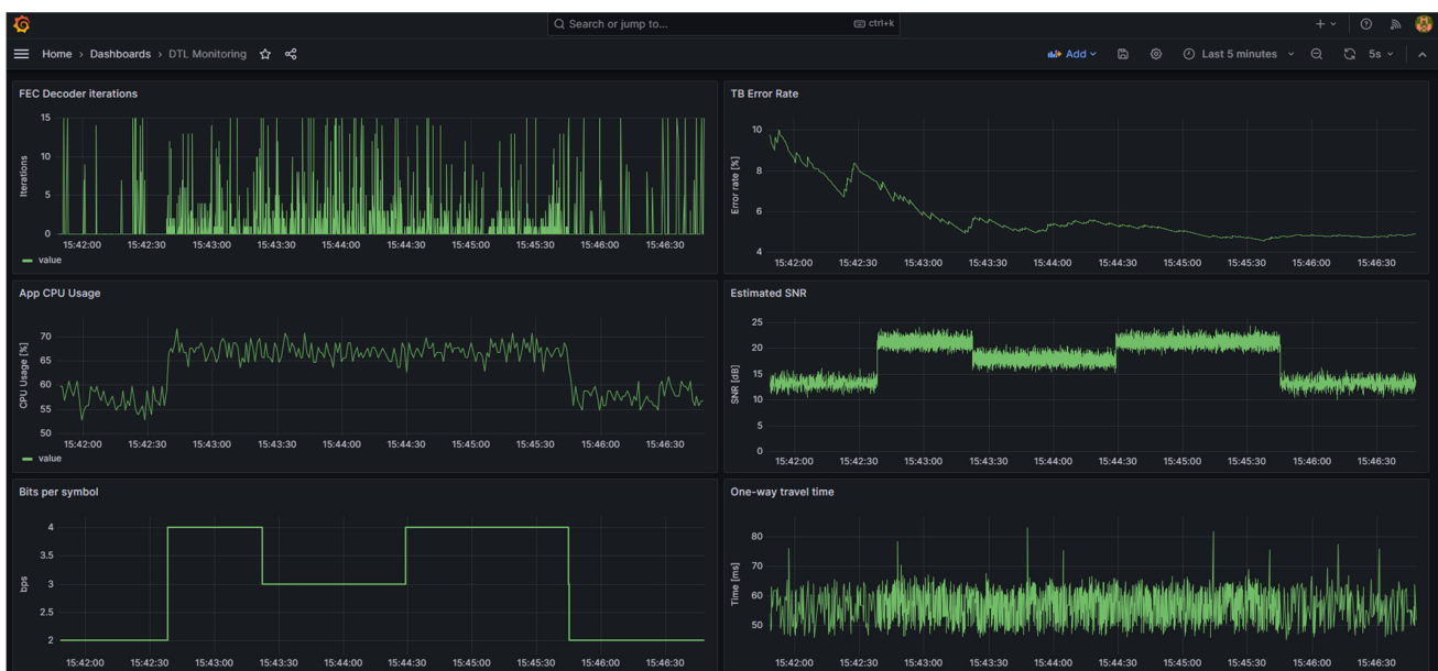
Figure 20. Evolution in time of some parameters of the tested adaptive OFDM transmission system developed in GNU radio.
