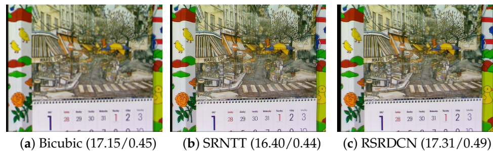
Figure 5. The reconstructed images of the first frame of Vid4's calendar clip. The values are PSNR and SSIM.
