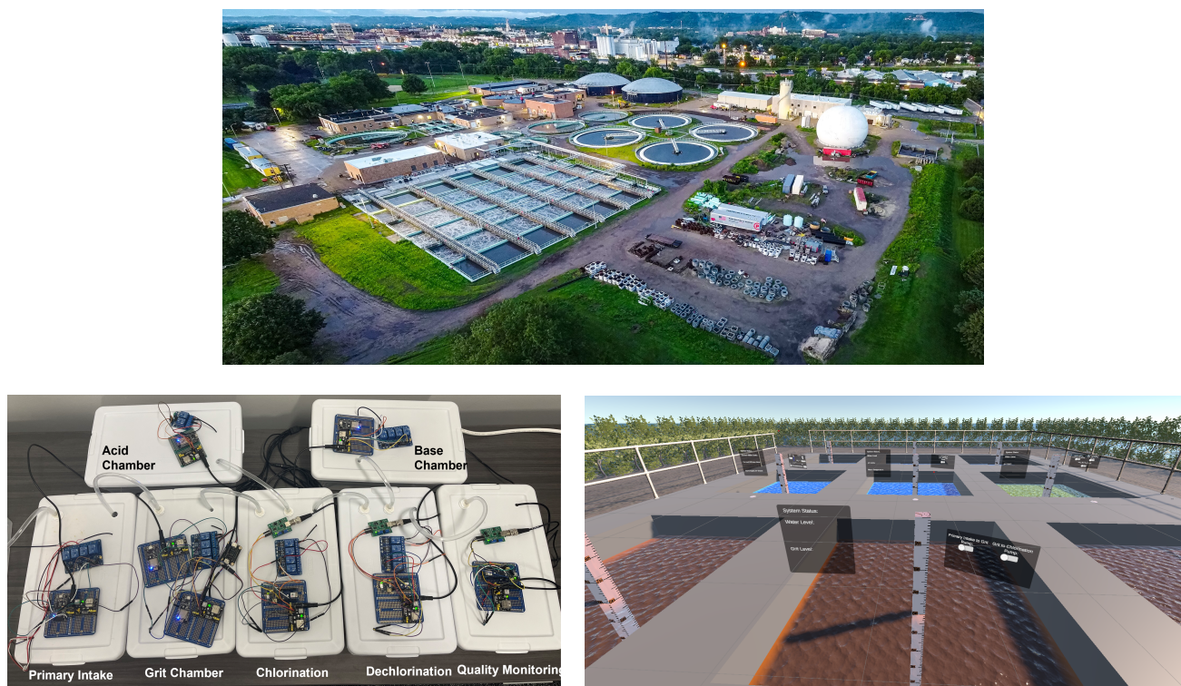
Figure 5. (Top) An aerial view of a water treatment facility in Wisconsin [79]. (Bottom Left) The hardware of the developed digital twin wastewater treatment facility. (Bottom Right) The VR interface of the developed digital twin wastewater treatment facility.
