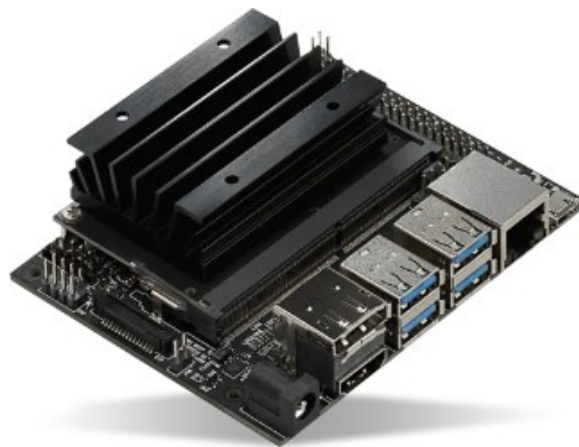
Figure 3. Nvidia Jetson Nano.
