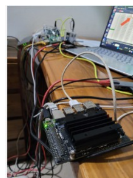
(b) Nvidia-Raspberry Pi Cluster
