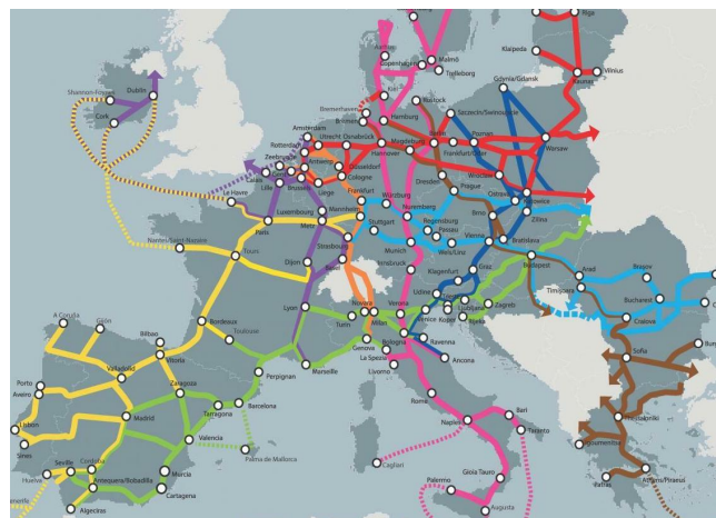
Figure 2. The “Trans-European Transport Network”, a critical infrastructure spanning the EU. The bold lines of different colors represent different “Corridors”; Yellow lines indicate the Atlantic corridor. Green lines indicate the Mediterranean corridor. Please see European Commission, Department of Mobility and Transport, Transport Themes ( https://transport.ec.europa.eu/transport-themes/infrastructure-and-investment_en , accessed on 1 March 2024).
