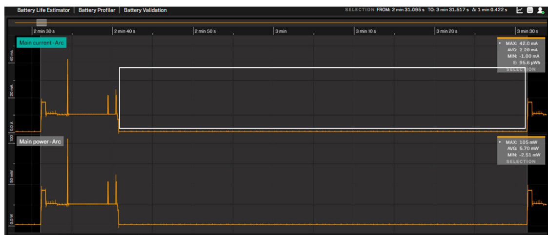
Figure 13. Complete energy profile of the IoT including the deep sleep time T_5 .
