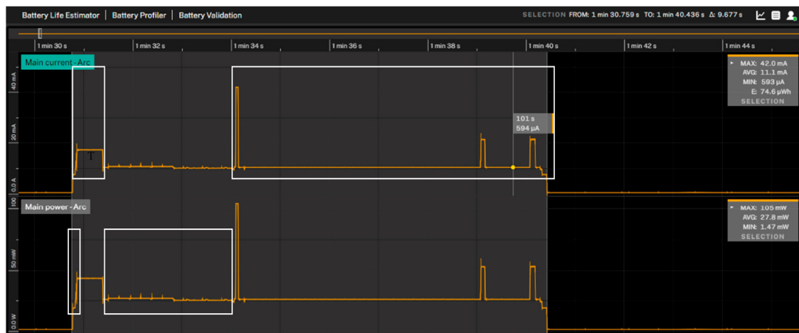
Figure 12. Energy profile of the IoT + vibration sensor from T_1 to T_4 . With a total duration of 9.66 s.
