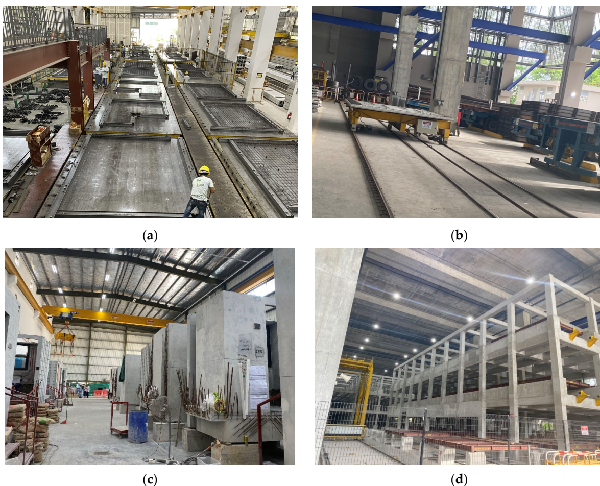
Figure 1. ICPH main facilities: (a) carousel system; (b) pallet circulation system; (c) modular fitting out; (d) robotic warehousing system (photos taken by Chen Chen in Singapore ICPHs).
