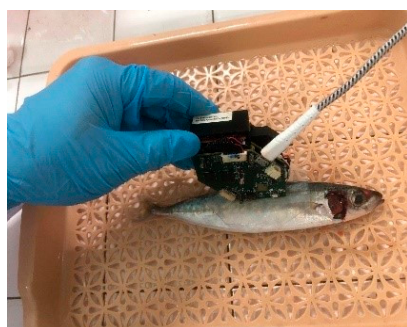
Figure 2. NIR spectrum measurement on a fish's body.
