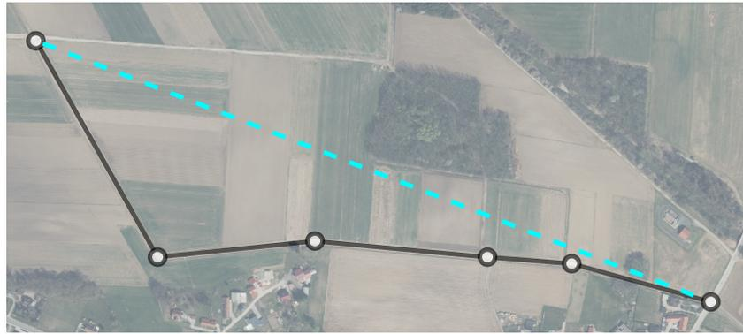
**Figure 9.** Distances between OpenStreetMap nodes versus straight-line distance between two nodes (intersections) (background source: [31]).
