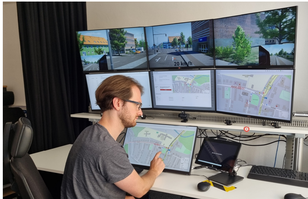
Figure 1. Remote operation center simulator together with the study set-up. The tablet on the bottom right was used for presentation of the secondary task.
