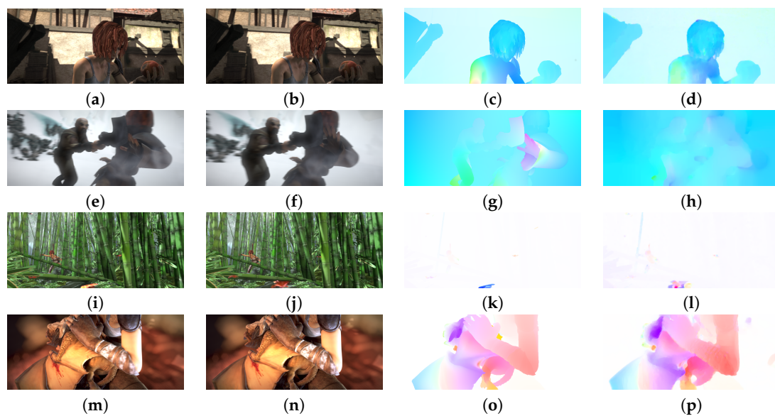
Figure 13. Image sequences used to estimate model parameters. In the parameter estimation, we used the first two frames of each considered sequence: (a–d) the frames of the alley_1 sequence, the ground truth, and our results, respectively. (e,f) the ambush_2 sequence, (g) the ground truth, and (h) our result. (i,j) frames of the bamboo_2 sequence, (k) the ground truth, and (l) our result. (m,n) the frame of bandage_1 sequence (o) the ground truth, and (p) our results.
