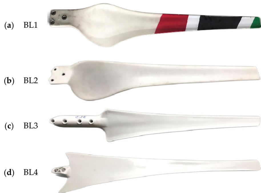
Figure 3. Rotor turbine blades with different shapes: (a) BL1; (b) BL2; (c) BL3; and (d) BL4.
