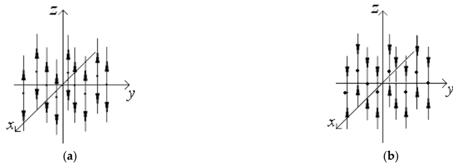
Figure 3. Schematic representation of the topology of the phase space of system (9) in the vicinity of the composed singular point of codimension 2: (a)—“unstable stationary plane”, (b)—“stable stationary plane”.
