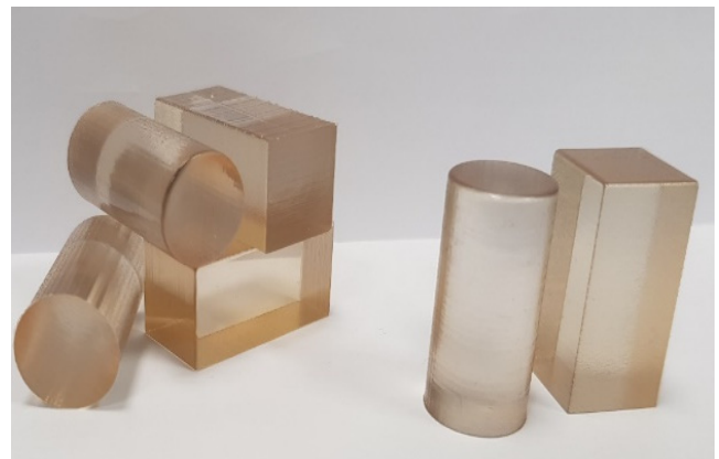
Figure 5. Standard solid samples drawn in x -, y -, and z -, directions and 3D-printed in the z -direction. Lines represent the build layers' direction [8].
