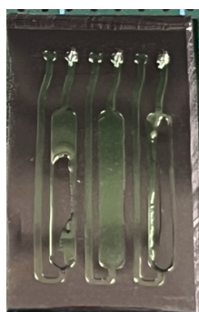
Figure S1. Collapsed microfluidic chips after being pressed at 0.5 MPa. The inner surface of the reaction channel was incorrectly bonded with the silicon base.
