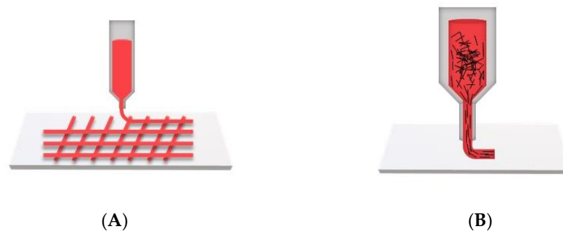
Figure 5. Schematics of 3D printing techniques for fiber alignment: (A) direct depositing of aligned and complex architecture scaffolds; (B) shear-induced alignment in the scaffold.
