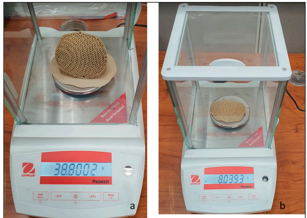
Figure 9. Weight scale reading of PEEK porous implant with (a) supports and (b) without supports.
