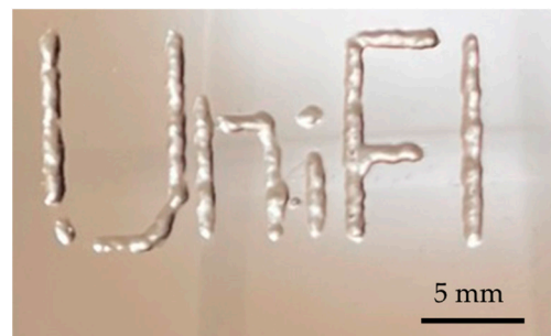
Figure 4. Example of a structure 3D printed with the GelMA-XG hydrogel.
