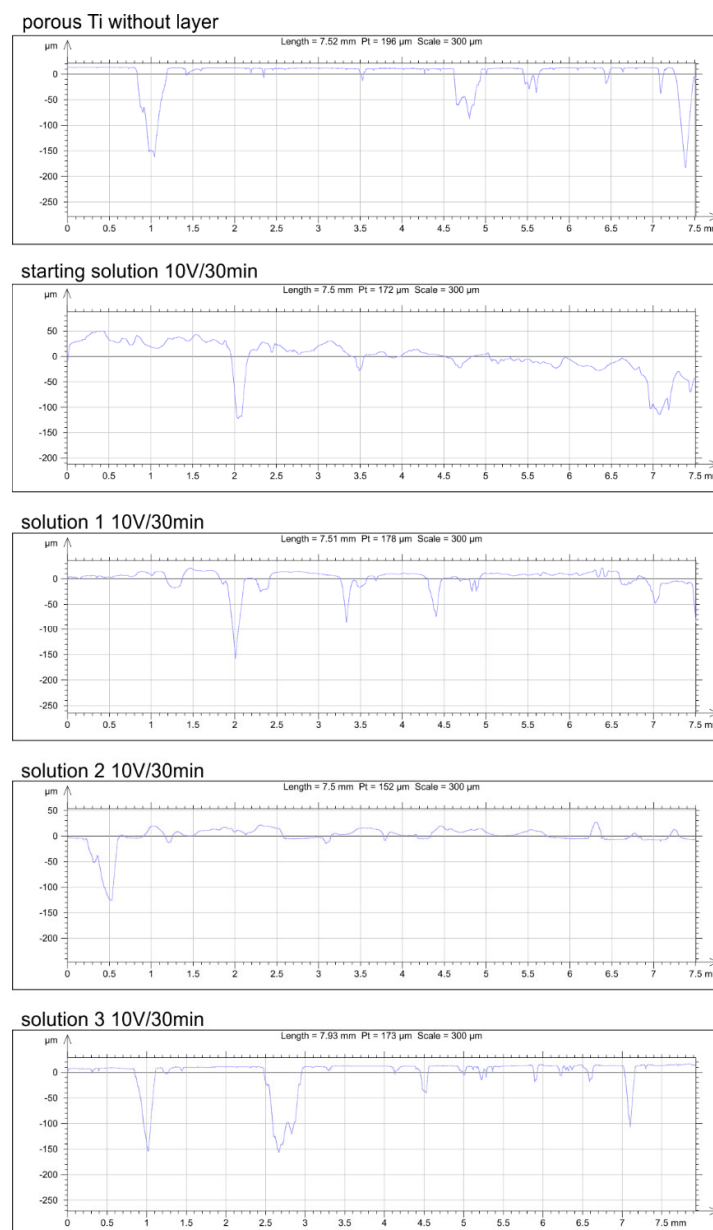
Figure 10. The roughness profile of porous Ti and chitosan coatings obtained at 10 V for 30 min from different solutions.
