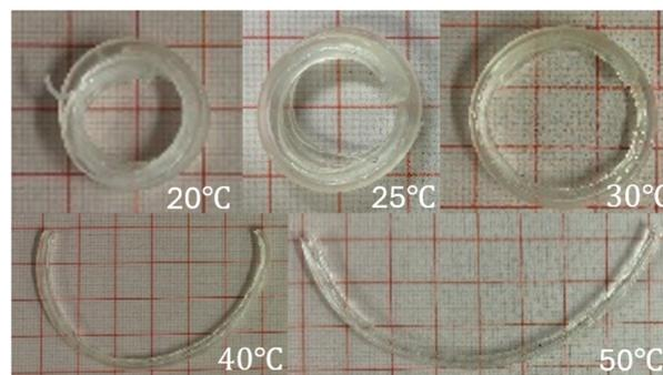
**Figure 7.** Swollen 100C sample at various temperatures.
