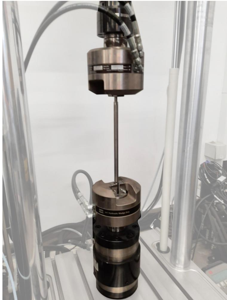
**Figure 5.** Implant positioning in clamps during the static torsion test.
