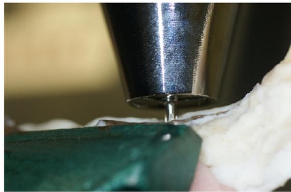
**Figure 8.** Removal torque measurement using a torque gauge.
