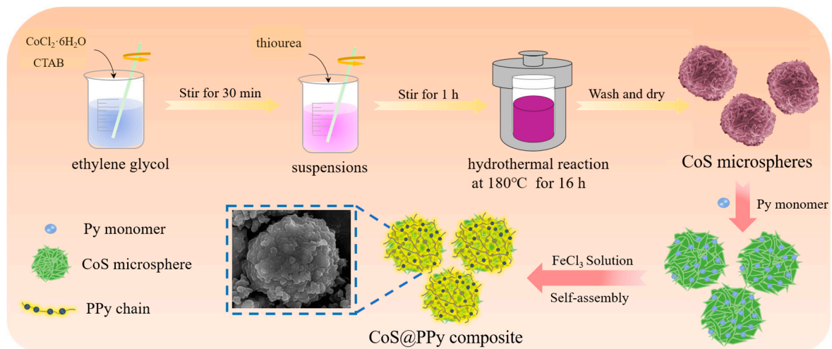
Figure 1. Schematic diagram of preparation process of CoS@PPy composites.
