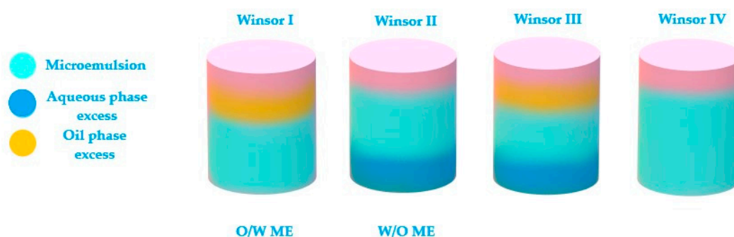
Figure 6. Schematic representation of Winsor phases I, II, III and IV, explaining the transition of phases from Winsor phase I to Winsor phase IV to obtain an ideal system.
