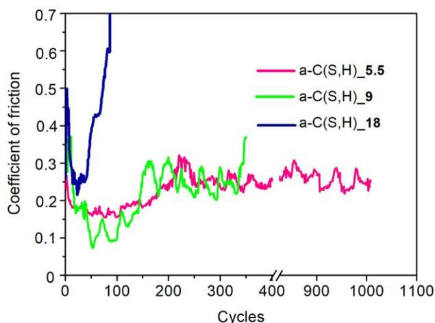
**Figure S10.** Characteristic evolution of the friction coefficient as a function of the cycle number for a-C(S,H) thin-film coatings obtained by reactive PLD at the pressures of H<sub>2</sub>S gas of 5.5, 9 and 18 Pa. Pin-on-disk tribometer testing was conducted in dry friction conditions at -100 °C.
