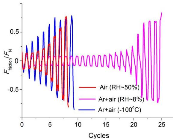
**Figure S4.** The friction force (in relation with the normal force) evolution during reciprocate sliding of the counterbody over the  $\text{MoS}_x$  coating under different environmental conditions. The  $\text{MoS}_x$  coating was obtained on the steel substrate by reactive PLD at  $\text{H}_2\text{S}$  pressure of 5.5 Pa.
