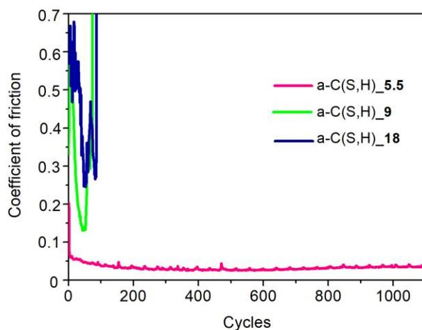
**Figure S8.** Characteristic evolution of the friction coefficient as a function of the cycle number for a-C(S,H) thin film coatings obtained by reactive PLD at the pressures of H<sub>2</sub>S gas of 5.5, 9, and 18 Pa. Pin-on-disk tribometer testing was conducted in dry friction conditions (air+Ar mixture, RH-8%) at 22 °C.
