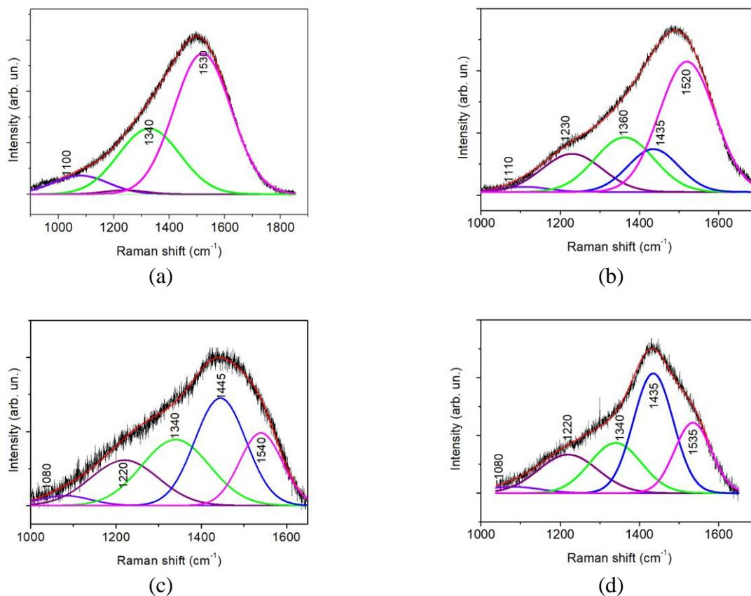
**Figure S3.** Raman spectra for (a) a-C(H) and (b–d) a-C(S,H) films obtained by PLD on Si substrate (a) under vacuum conditions and in reactive H<sub>2</sub>S gas at pressures of (b) 5.5, (c) 9, and (d) 18 Pa. The model of spectrum decomposition into the indicated peaks is discussed in the text of the article.
