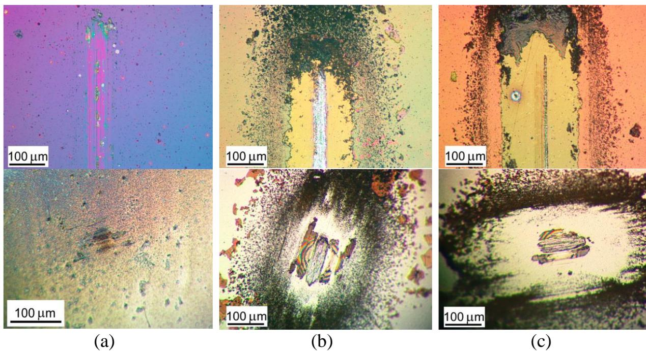
**Figure S9.** Optical images of wear tracks and wear scars formed on the steel substrates and steel balls for a-C(S,H) thin film coatings obtained by reactive PLD at the different pressures of H<sub>2</sub>S gas: (a) 5.5, (b) 9, and (c) 18 Pa. Pin-on-disk tribometer testing was conducted in dry friction conditions at 22 °C. The test durations are indicated in Figure S8.
