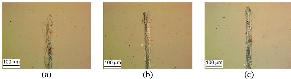
**Figure S5.** Optical images of wear tracks formed on the steel substrates for  $\text{MoS}_x$  thin-film coating obtained by reactive PLD at  $\text{H}_2\text{S}$  pressure of 5.5 Pa. Pin-on-disk tribometer testing was conducted in (a) wet friction conditions (RH~50%) at 22 °C, (b) dry friction conditions (RH~8%) at 22 °C, and (c) dry friction conditions at -100 °C. The test durations are indicated in Figure S4.
