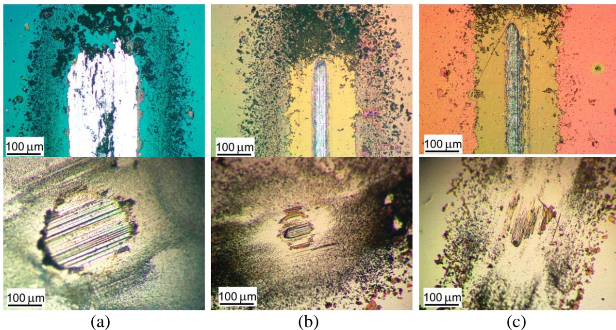
**Figure S7.** Optical images of wear tracks and wear scars formed on the steel substrates and steel balls for a-C(S,H) thin-film coatings obtained by reactive PLD at the different pressures of H<sub>2</sub>S gas: (a) 5.5, (b) 9, and (c) 18 Pa. Pin-on-disk tribometer testing was conducted in wet air (RH~58%) at 22 °C. The test durations are indicated in Figure S6.
