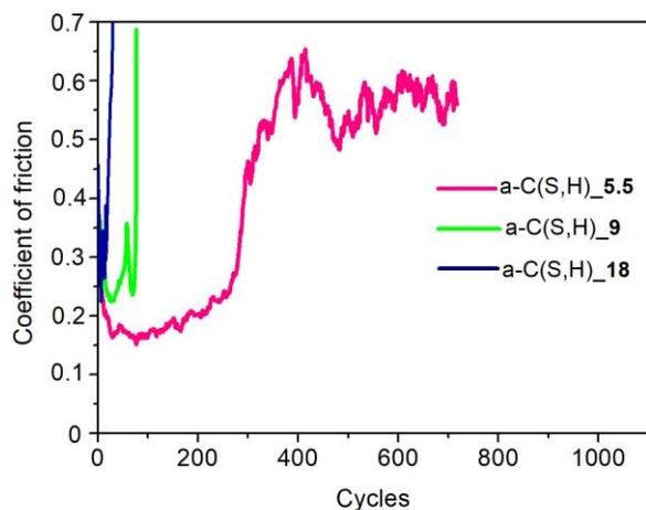
**Figure S6.** Characteristic evolution of the friction coefficient as a function of the cycle number for a-C(S,H) thin-film coatings obtained by reactive PLD at the pressures of H<sub>2</sub>S gas of 5.5, 9 and 18 Pa. Pin-on-disk tribometer testing was conducted in wet air (RH~58%) at 22 °C.
