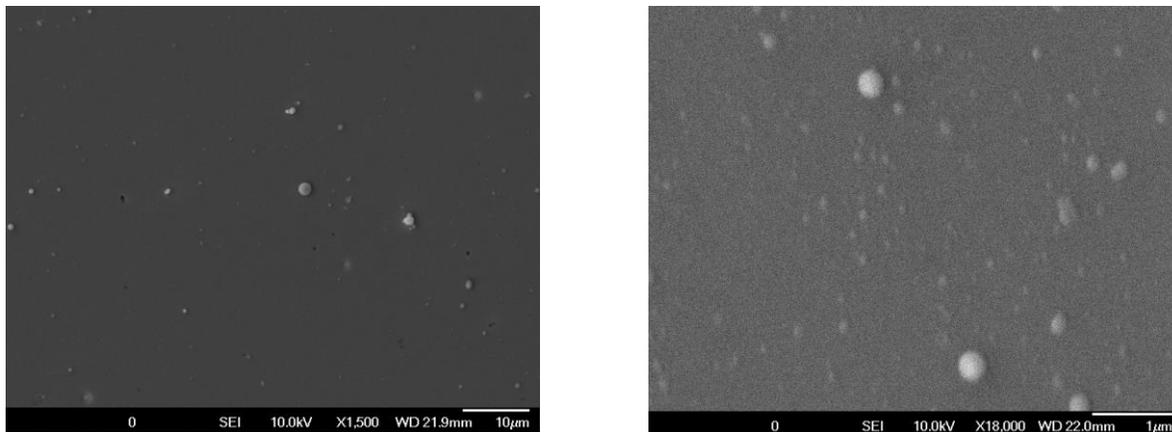
**Figure S2.** Typical SEM images (two magnifications) of a-C(S, H) film obtained on a steel substrate by reactive PLD in H<sub>2</sub>S.
