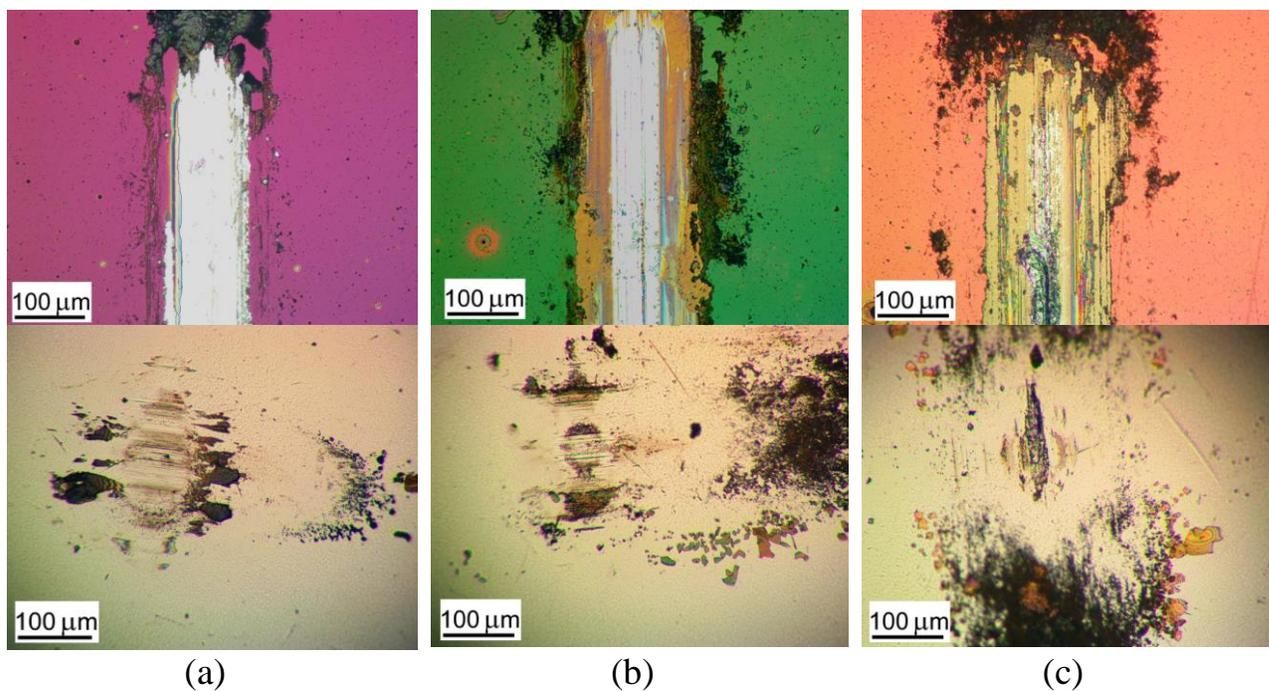
**Figure S11.** Optical images of wear tracks and wear scars formed on the steel substrates and steel balls for a-C(S,H) thin-film coatings obtained by reactive PLD at the different pressures of H<sub>2</sub>S gas: (a) 5.5, (b) 9, and (c) 18 Pa. Pin-on-disk tribometer testing was conducted in dry friction conditions at -100 °C. The test durations are indicated in Figure S10.
