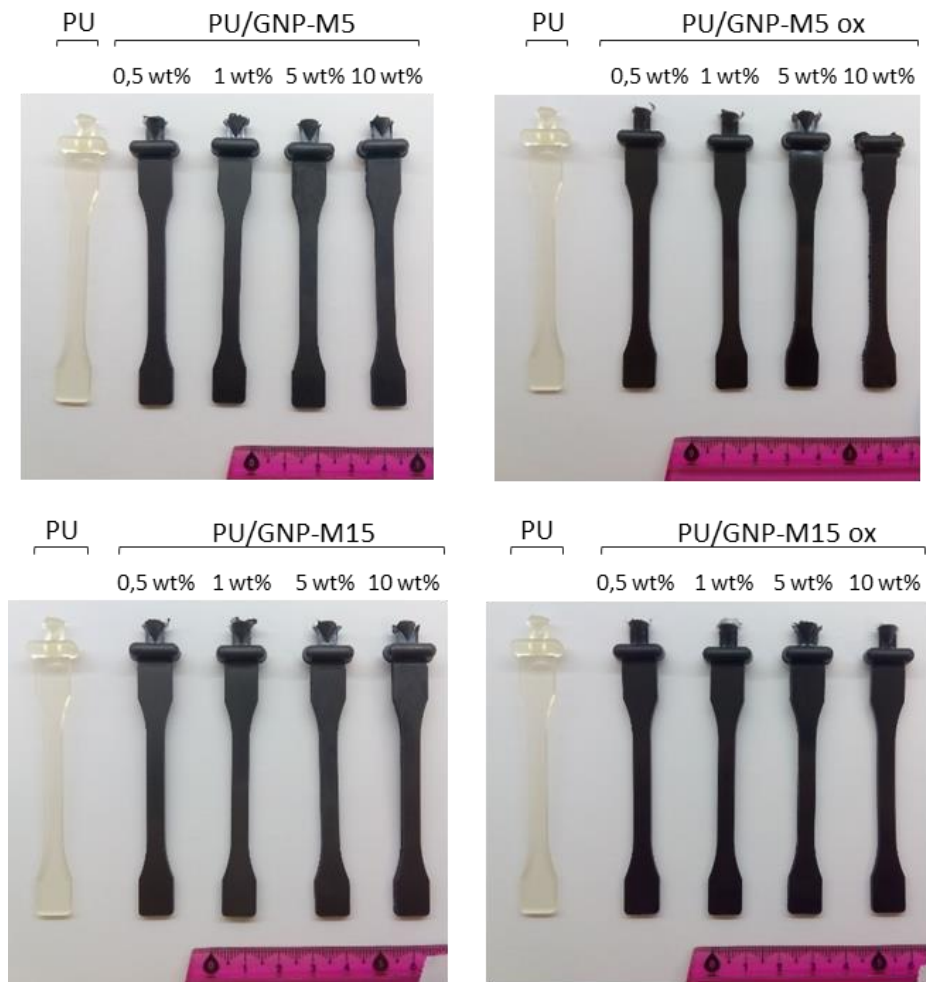
Figure S1. Images of the PU and PU/GNP composites produced by melt-blending after injection molding.
