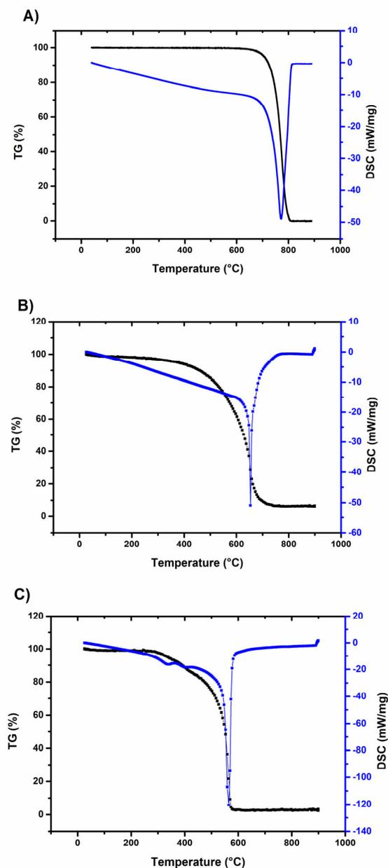
**Figure S3.** TGA (left Y-axis) and TGA (right Y-axis) curves recorded for C-BNM under oxygen atmosphere with a heating rate of 10 K/min
