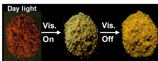
Figure S10. Photographs of the AA-CDs-2 powder at ambient conditions under day light, and visible (Vis.) light LED ( \lambda_{em}=420 nm) on and just being switched off, respectively.
