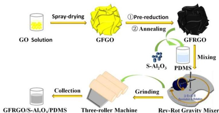
Figure 1. Scheme for the preparation of GFRGO/S-Al<sub>2</sub>O<sub>3</sub>/PDMS composites.
