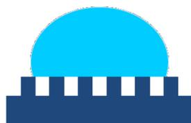
**Figure 4.** The Cassie model presumes that in the grooves, the air is trapped below the liquid droplet resulting in a composite solid to liquid-to-vapor interface.
