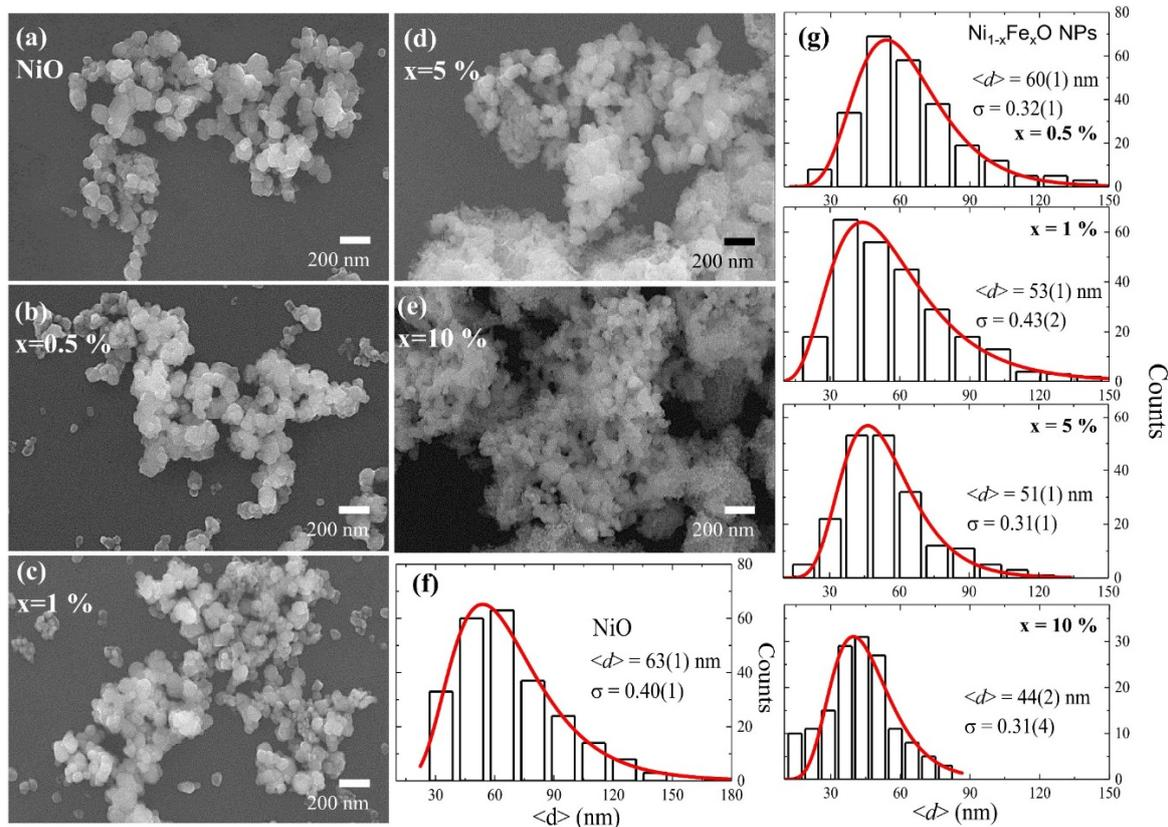
**Figure 1.** (a–e) SEM images of NiO, 0.5, 1, 5 and 10% samples, respectively. Histogram obtained from (f) NiO, (g) 0.5, 1, 5, and 10% samples (top to bottom). The solid red lines represent a fit using the Log-normal distribution function.
