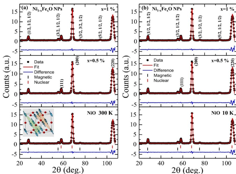
**Figure 2.** The Rietveld refined (red line) neutron powder diffraction (NPD) spectra (dots) from NiO, 0.5, and 1% samples (bottom to top) taken at (a) 300 K and (b) 10 K are calculated with  $Fm\bar{3}m$  symmetry. The blue line represents the difference between experimental and fitted spectra. The vertical black and short red lines represent the magnetic and nuclear brags reflection positions. Inset in the bottom panel of (a): a unit cell of NiO with two magnetic sublattices.
