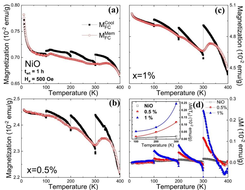
**Figure 6.** The FC magnetic memory effect from (a) NiO, (b) 0.5%, and (c) 1% samples. (d) The difference in magnetization  $\Delta M = M_{FC}^{cool} - M_{FC}^{mem}$  concerning temperature. The value of maximum  $\Delta M(T_S)$  at each stopping temperature,  $T_S$  is given in the inset of a figure (d).
