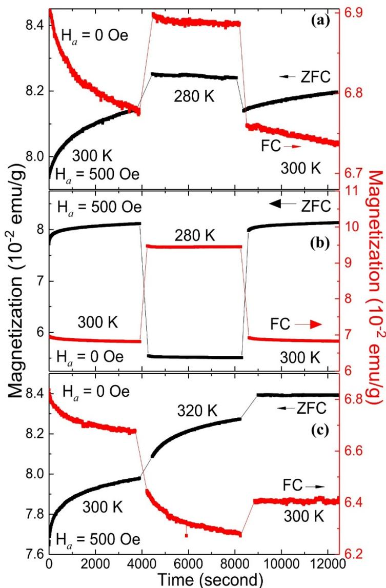
**Figure 7.** The effect of temperature-cooling (a) without (b) with field switching and (c) temperature-heating cycle without field switching during ZFC and FC magnetization relaxation from 1% sample.
