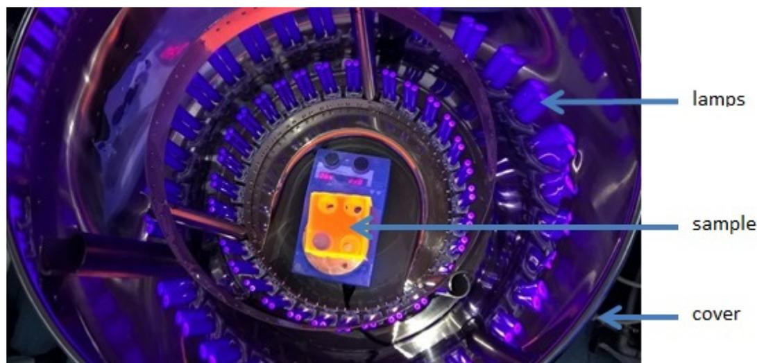
**Figure 1.** The interior of a photoreactor constructed by our team.
