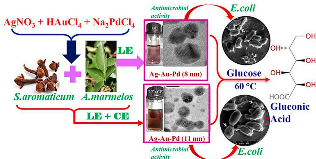
**Figure 7.** Schematic illustration of the fabrication of trimetallic NPs and their catalytic activities in the glucose oxidation and/or antimicrobial applications. Reproduced from [88], with permission from American Chemical Society, 2015.
