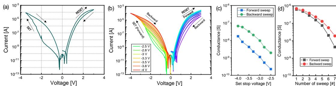
**Figure 2.** Current-voltage (I–V) curves and multilevel conductance characteristics of TiN/Ti/TiO<sub>2</sub>/SiO<sub>x</sub>/Si device: (a) typical I–V curves; (b) current change characteristics by repeated sweep from  $-2.5$  to  $-4$  V for set process and fixed 3 V for reset process; (c) conductance gradually increases with incremental set stop voltage; (d) conductance gradually decreases using the same voltage sweep (3 V).
