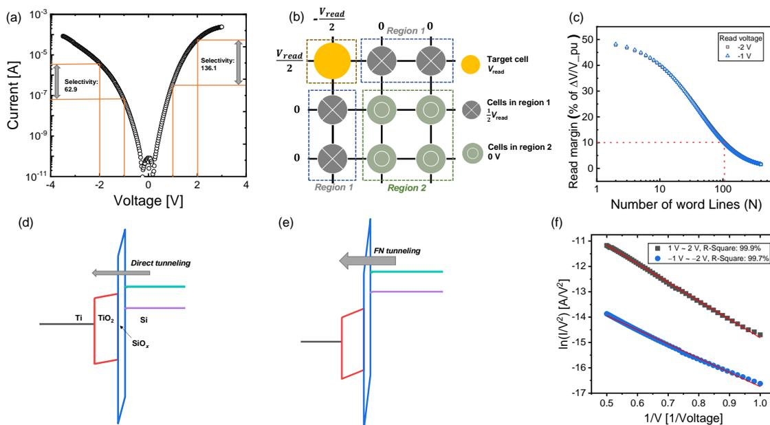
**Figure 7.** Nonlinear characteristics of TiN/Ti/TiO<sub>2</sub>/SiO<sub>x</sub>/Si device: (a) I–V curve with high selectivity in LRS pulse schemes; (b) half-bias scheme in cross-point array structure; (c) read margin as a function of number of word lines; energy band diagrams at (d) low voltage and (e) high voltage; (f)  $\ln(I/V^2)$  versus  $1/V$  plot for Fowler–Nordheim (FN) tunnel fitting.
