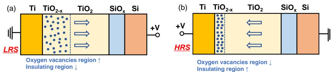
**Figure 3.** Illustration of a simple oxygen vacancy model to explain the conductance change of Ti/TiO<sub>2</sub>/SiO<sub>x</sub>/Si device in (a) low-resistance state (LRS) and (b) high-resistance state (HRS). Oxygen vacancies are full circles with blue color and the arrows indicate the moving direction of oxygen ions.
