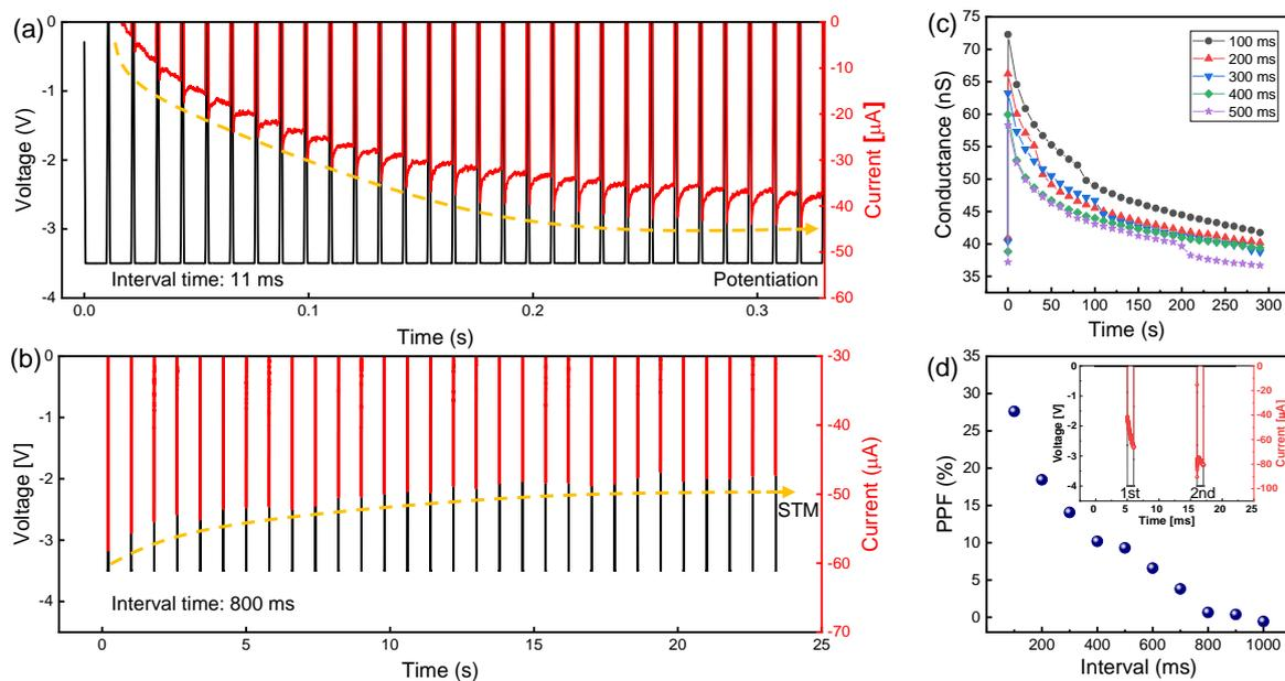
**Figure 5.** Short-term dynamics of TiN/Ti/TiO<sub>2</sub>/SiO<sub>x</sub>/Si device: (a) current was maintained by a short time interval (11 ms) after the set process; (b) current decayed from LRS in a long time interval (800 ms); (c) conductance decayed after 5 consecutive pulses were applied as a function of the time interval between pulses; (d) paired-pulse facilitation (PPF) as a function of interval time between paired pulses.
