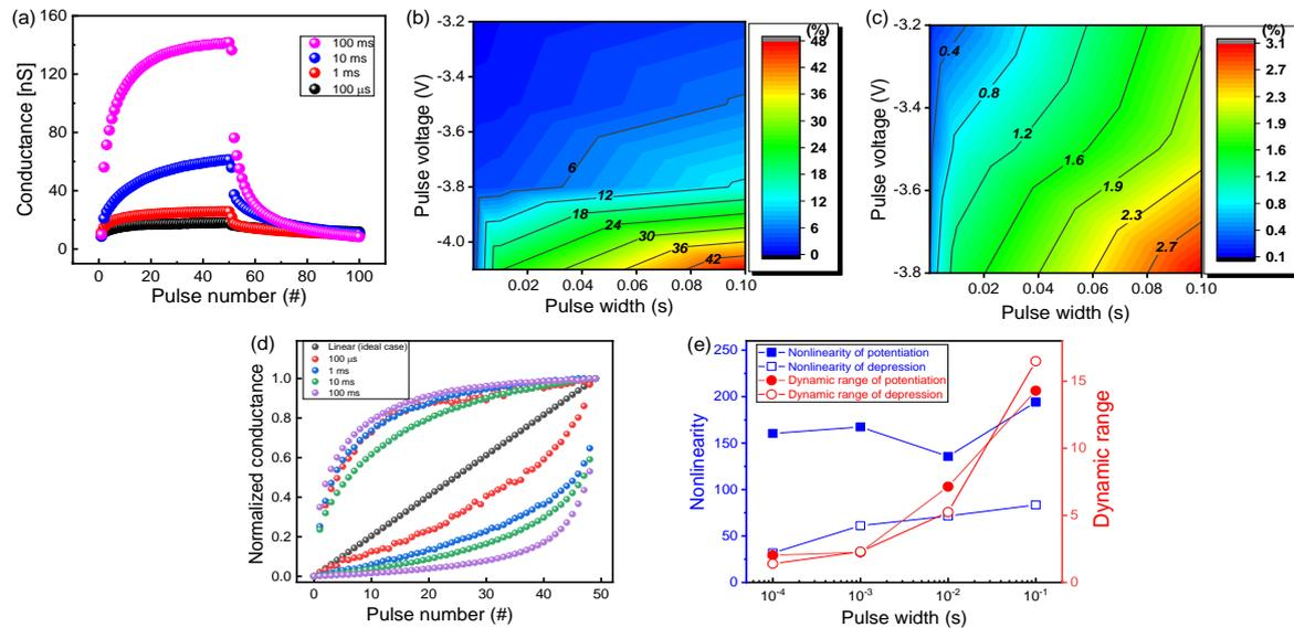
**Figure 4.** Potentiation and depression characteristics of TiN/Ti/TiO<sub>2</sub>/SiO<sub>x</sub>/Si device: (a) Pulse-width-controlled conductance change; contour maps of (b) potentiation and (c) depression as a function of pulse voltage and width; (d) normalized conductance in different pulse widths; (e) nonlinearity and dynamic range as a function of pulse width.
