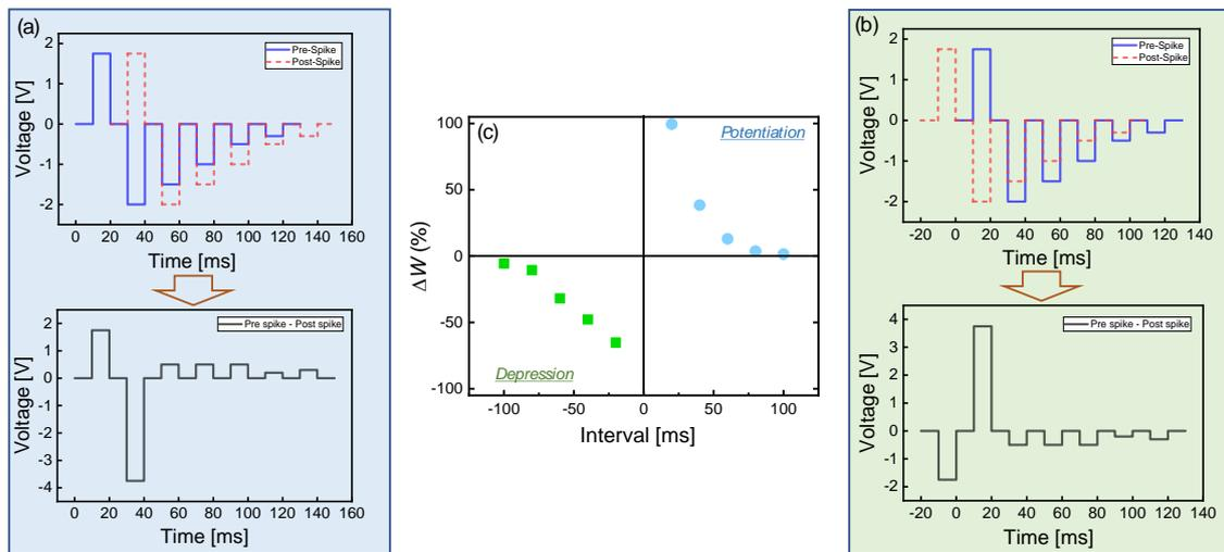
**Figure 6.** Spike-timing-dependent plasticity (STDP) of TiN/Ti/TiO<sub>2</sub>/SiO<sub>x</sub>/Si device: pulse schemes (pre- and postspike pulse trains) for (a) potentiaon and (b) depression; (c) STDP-like curve including potentiation and depression as a function of interval timing.
