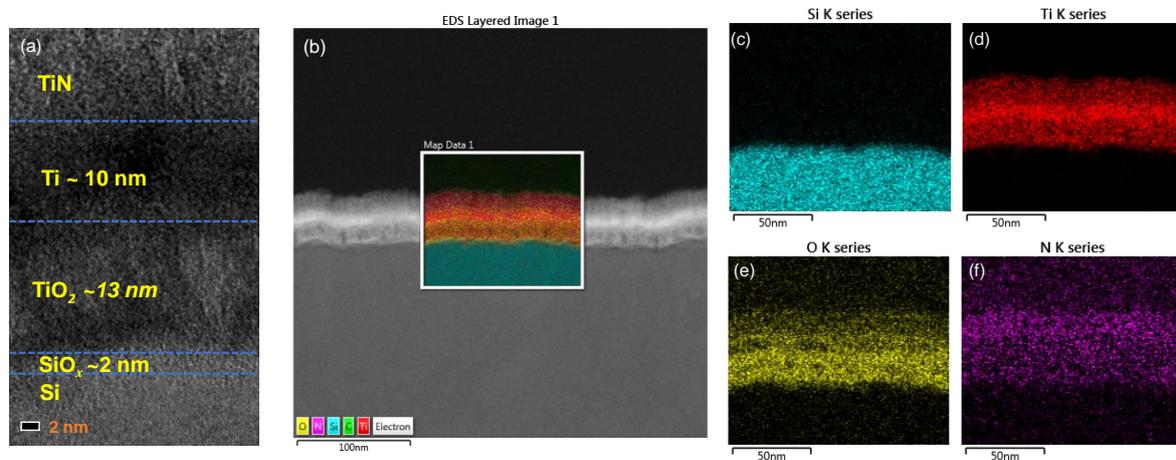
**Figure 1.** (a) TEM image TiN/Ti/TiO<sub>2</sub>/SiO<sub>x</sub>/Si device; (b) energy-dispersive X-ray spectroscopy (EDS) layered image in scanning transmission electron microscope (STEM); each element ((c) Si, (d) Ti, (e) O, (f) N) of TiN/Ti/TiO<sub>2</sub>/SiO<sub>x</sub>/Si device.
