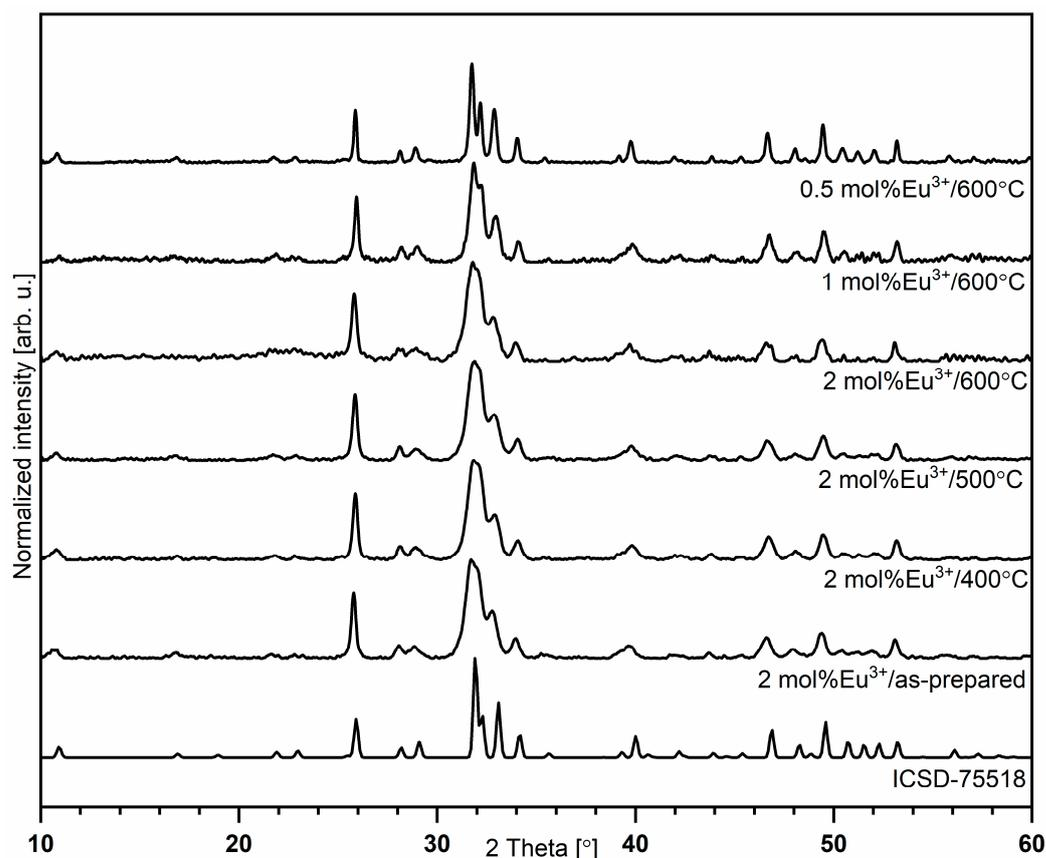
**Figure 1.** X-ray diffraction pattern of silicate-substituted hydroxyapatite co-doped with 2 mol% Sr<sup>2+</sup> and x mol% Eu<sup>3+</sup> ions.
