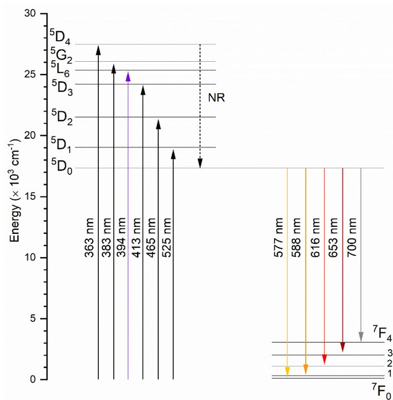
Figure 6. The simplified energy level scheme for  $\text{Eu}^{3+}$  ion in silicate-substituted strontium-doped hydroxyapatite.
