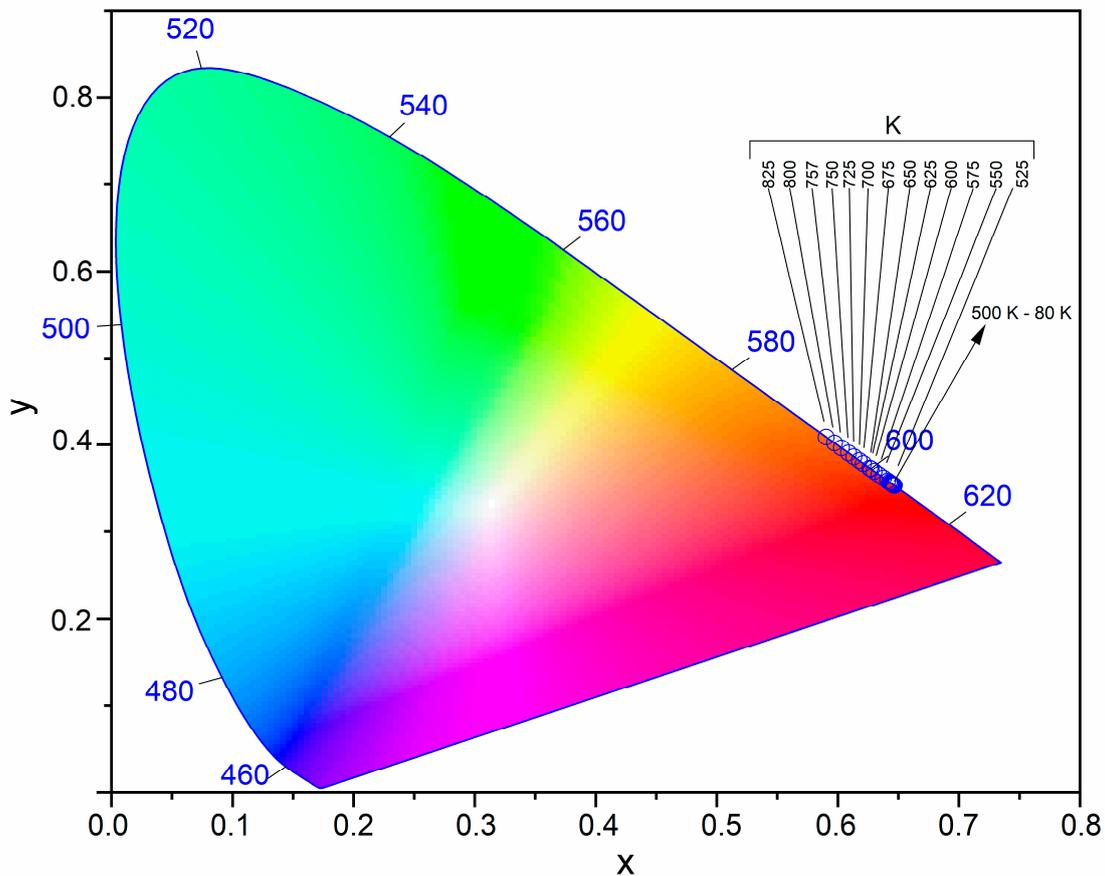
Figure 8. CIE 1931 chromaticity diagram of the  $\text{Ca}_{9.6}\text{Sr}_{0.2}\text{Eu}_{0.2}(\text{PO}_4)_2(\text{SiO}_4)_4(\text{OH})_2$  as a function of ambient temperature.
