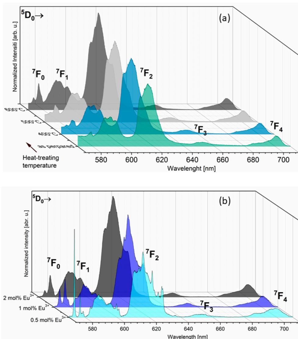
**Figure 4.** Emission spectra of Ca<sub>9.6</sub>Sr<sub>0.2</sub>Eu<sub>0.2</sub>(PO<sub>4</sub>)<sub>2</sub>(SiO<sub>4</sub>)<sub>4</sub>(OH)<sub>2</sub> as a function of sintering temperature (a) and Ca<sub>9.8-x</sub>Sr<sub>0.2</sub>Eu<sub>x</sub>(PO<sub>4</sub>)<sub>2</sub>(SiO<sub>4</sub>)<sub>4</sub>(OH)<sub>2</sub>, where x = 0.5, 1.0, 2.0 mol%, sintered at 600 °C (b).
