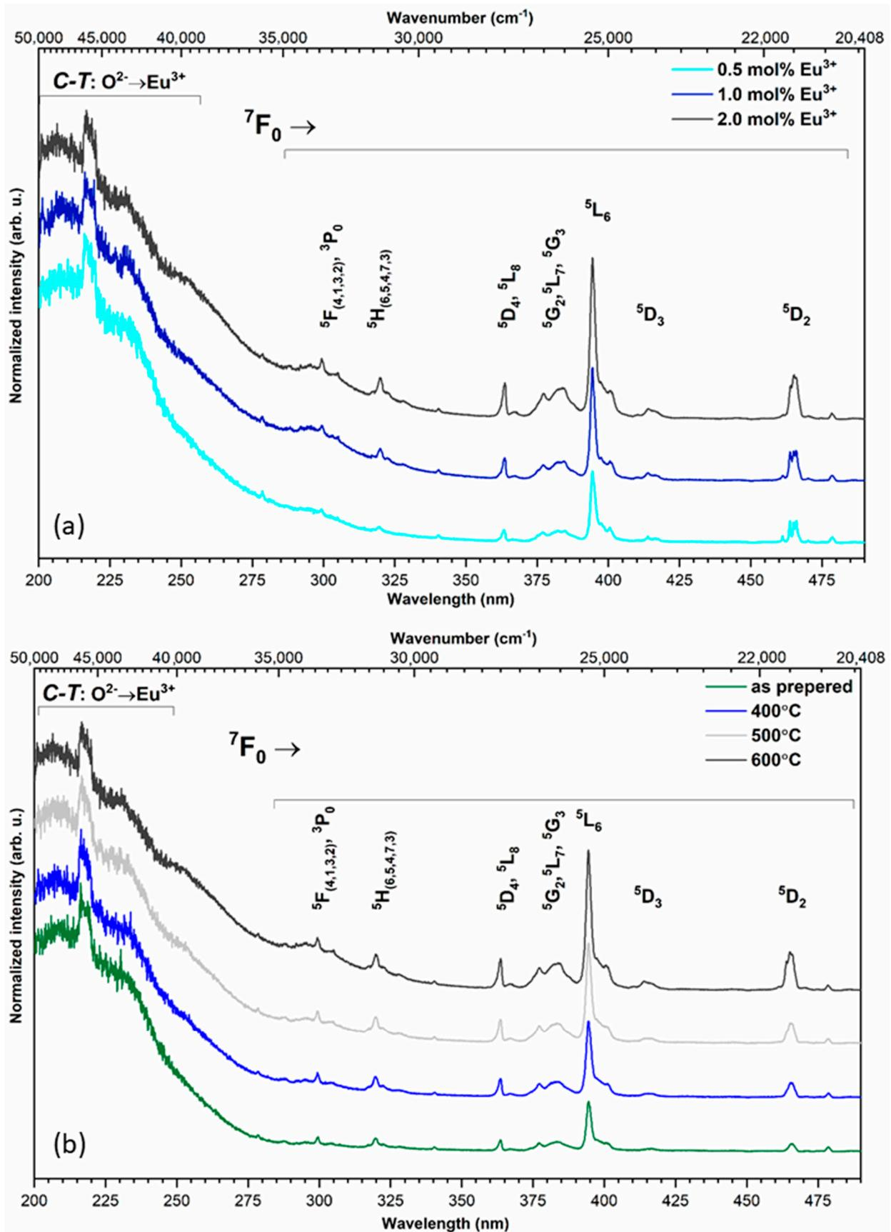
**Figure 3.** Excitation emission spectra of Ca<sub>9.8-x</sub>Sr<sub>0.2</sub>Eu<sub>x</sub>(PO<sub>4</sub>)<sub>2</sub>(SiO<sub>4</sub>)<sub>4</sub>(OH)<sub>2</sub>, where x = 0.5, 1.0, 2.0 mol%, sintered at 600 °C (a) as well as Ca<sub>9.6</sub>Sr<sub>0.2</sub>Eu<sub>0.2</sub>(PO<sub>4</sub>)<sub>2</sub>(SiO<sub>4</sub>)<sub>4</sub>(OH)<sub>2</sub> as a function of sintering temperature (b).
