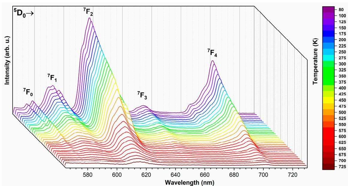
Figure 7. Temperature-dependent emission spectra of the  $\text{Ca}_{9,6}\text{Sr}_{0,2}\text{Eu}_{0,2}(\text{PO}_4)_2(\text{SiO}_4)_4(\text{OH})_2$ , sintered at  $600^\circ\text{C}$ .
