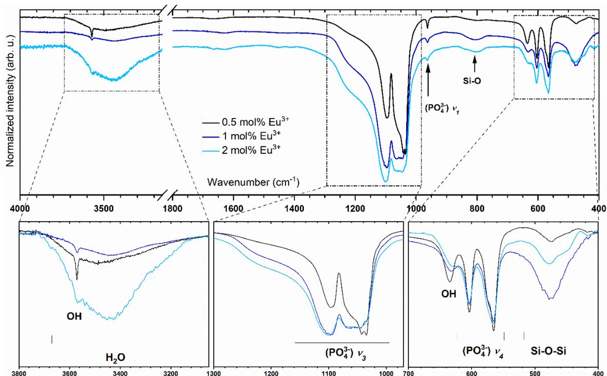
**Figure 2.** FT-IR spectra of the silicate-substituted hydroxyapatite co-doped with  $\text{Sr}^{2+}$  (2.0 mol%) and  $\text{Eu}^{3+}$  (0.5, 1.0 and 2.0 mol%) ions.
