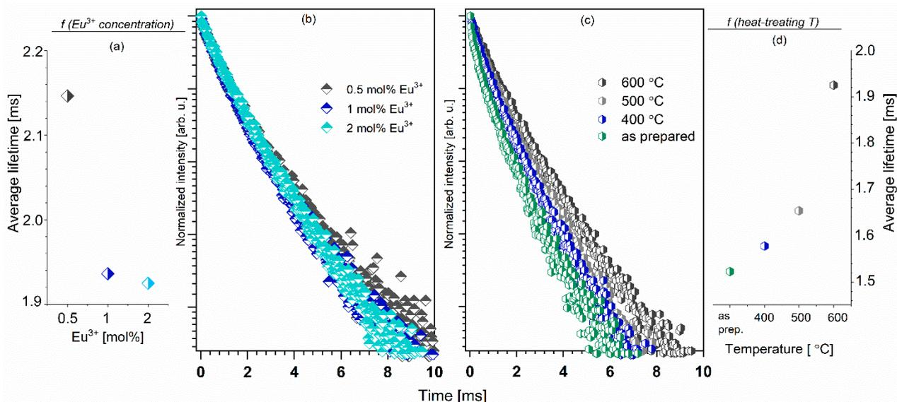
**Figure 9.** Calculated average lifetimes (a) as well as luminescence decay profiles (b) of  $\text{Ca}_{9.8-x}\text{Sr}_{0.2}\text{Eu}_x(\text{PO}_4)_2(\text{SiO}_4)_4(\text{OH})_2$ , sintered at 600 °C, as a function of  $\text{Eu}^{3+}$  ion concentration. Luminescence decay profiles (c) and calculated average lifetimes (d) of the  $\text{Ca}_{9.6}\text{Sr}_{0.2}\text{Eu}_{0.2}(\text{PO}_4)_2(\text{SiO}_4)_4(\text{OH})_2$  as a function of sintering temperature.
