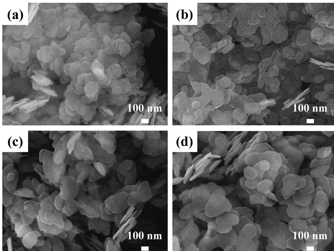
**Figure S2.** Scanning electron microscope image of (a) Ga@LDH-1, (b) Ga@LDH-3, (c) Ga@LDH-6 and (d) Ga@LDH-12.
