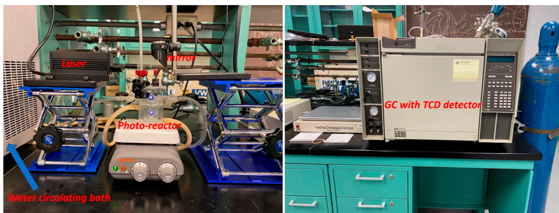
Figure S4. The picture of the experimental setup for the photocatalytic H 2 evolution.
