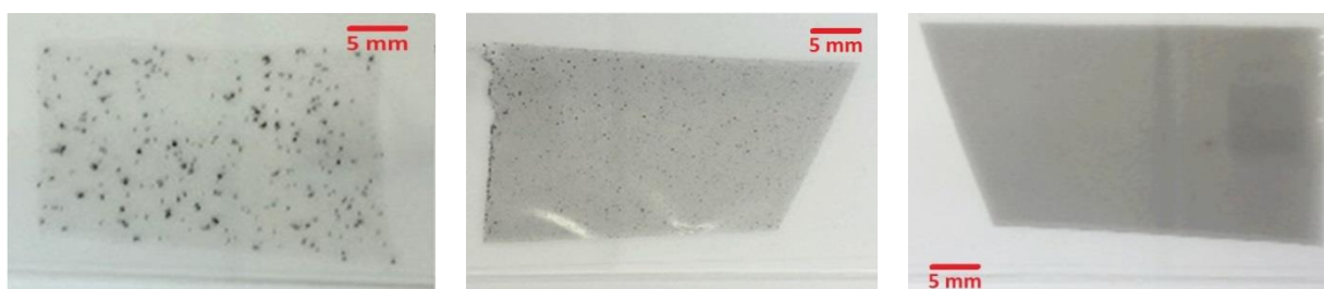
Figure 4. Dried films from preliminary study, without any secondary dispersion step. Left: 2.5 wt.% cellulose acetate (CA) solution (low viscosity), middle: 5 wt.% CA solution, right: 10 wt.% CA solution.
