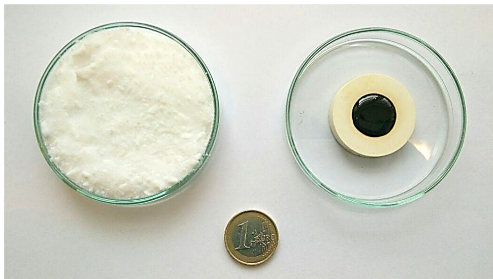
Figure 1. (left) Fumed silica nanoparticles and (right) the bitumen sample.
